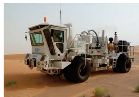
Sercel's new nomad 90 vibrator has improved manoeuvrability.
