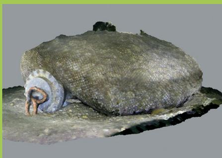
**Cover image:** A 3D model of a subsea "dry mate" electrical connector developed from underwater video cameras and imagery by UK company Rovco. Rovco imagines a future where video images from underwater vehicles could be converted into 3D models in real time, leading to big improvements in how the ROV operations could be carried out. For more information see page 19
