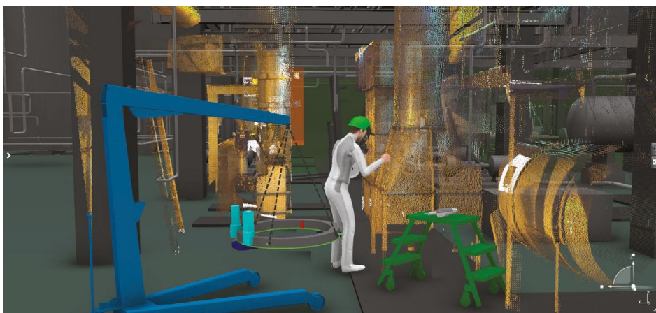
Doing decommissioning virtually - a virtual image of a plant within Dassault’s “3DEXPERIENCE” platform showing “Ergonomics At Work” functionality related to decommissioning
